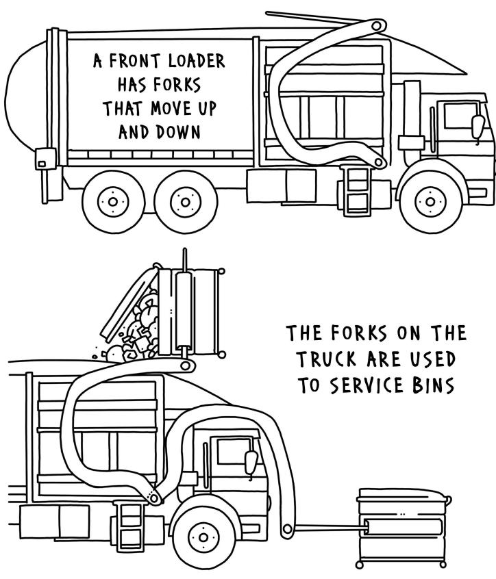
THE MATERIAL IS DUMPED INTO AN OPENING AT THE TOP OF THE TRUCK
